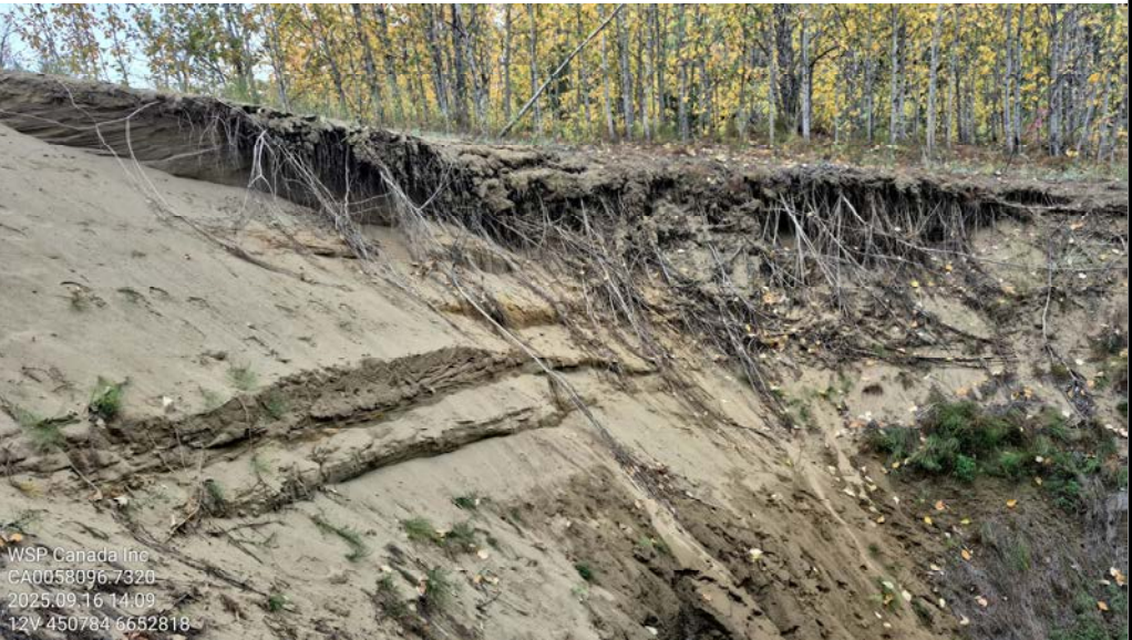
Photo 15 – headscarp with overhanging vegetation. Note the moist soil on the lower right and bedded sand structure at the crest and mid-photo banding.
